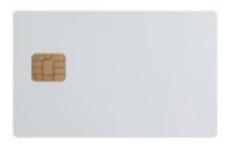
The SLE4428 is a standard, low-cost EEPROM memory smartcard with 1K bytes of available storage, an irreversible write protection feature and a 2-byte programmable security code.
